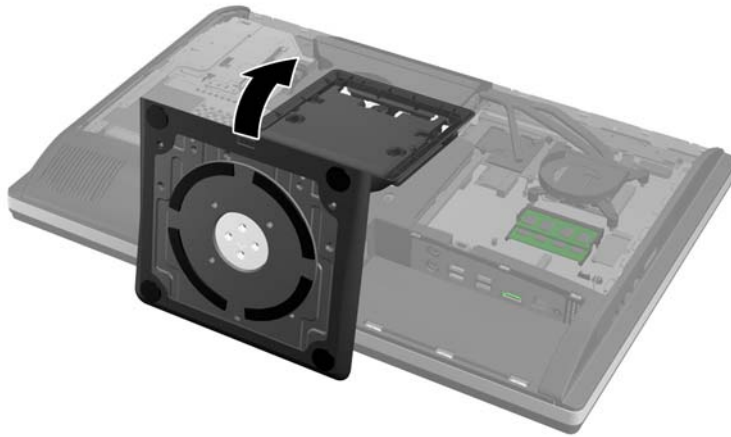
Figure 6-16 Removing the stand
